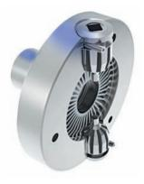
This cutaway image shows the unit's heavy-duty precision gear train. The mechanical advantage of the gears in combination with our unique double-angle expanding sleeves produces outstanding grip force on the workpiece.
